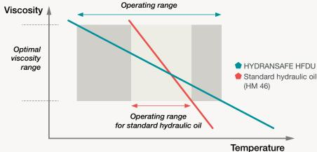
HYDRANSAFE HFDU is specifically formulated to offer an extended operating temperature range. The oil's cold and hot performance enable it to be used in a wide variety of applications.
