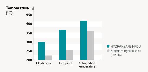
> HYDRANSAFE HFDU is a synthetic biodegradable oil with high fire resistance, offering optimal protection for equipments.
